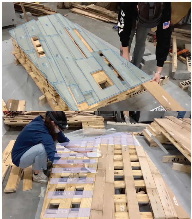
Figure 8. Mixed-reality guided laminating and gluing process.
